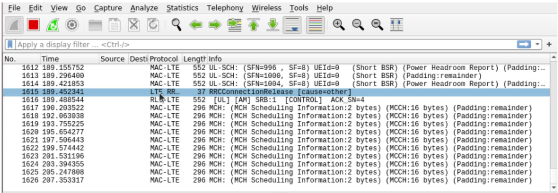
The image shows a screenshot of the Wireshark network traffic analysis tool. The main pane displays a list of captured packets. The selected packet (No. 1615) is an RRCConnectionRelease frame from the LTE RRC protocol. The other packets are MAC-LTE frames containing MCH Scheduling Information.
