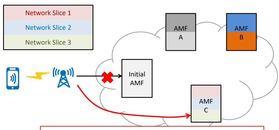
Select AMF C as Target AMF to service all Network Slice Re-allocate initial AMF to AMF C
