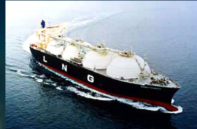
"Energy Frontier" Capacity: 147,591 m 3 Length: 289.53 m Width: 49.00 m Draft: 11.40 m
